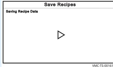
The "Save Recipes" screen appears during the saving process. When the process is complete, the "USB Functions" screen appears.
