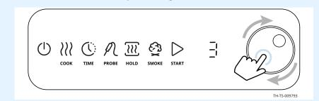
5. On double cavity ovens only, **turn** the knob to select the cavity to save the recipe to (top, bottom, or both).
